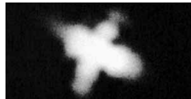
Figure 5 The appearance of a point object due to the presence of astigmatism. Compare with Figure 3.
