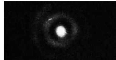
Figure 4 The appearance of the Airy disk when spherical aberration is present. Photomicrograph taken with a 4 mm, 0.65 N.A. objective, purposely spaced incorrectly to show the effect of lens spacing on spherical aberration. Compare with Figure 3.
